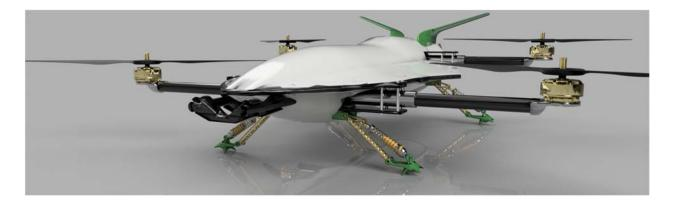
V2.0 is a complete redesign which lowers manufacturing costs and increases output capacity by reducing build times. A lifting body was added to V2.0 to aid in the efficiency of flight time and to reduce drag, weight and unnecessary parts.
